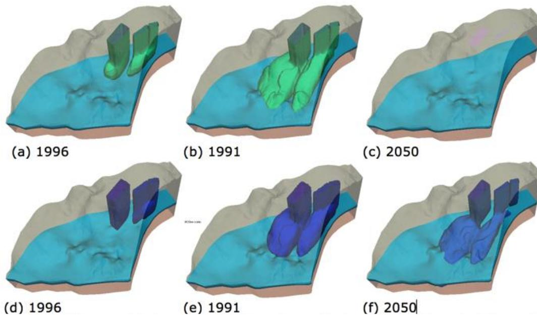
Figure 3. The simulated evolution of (a-c) low-pH plume ( $\text{pH} > 4$ ) and (d-f) uranium plume (concentration  $> 1 \times 10^{-6} \text{ mol/L}$ ). The sky blue region is the low permeable TCCZ, which separates the upper and lower aquifers. Vertical exaggeration = 15X.
