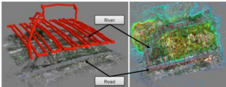
Figure 2 Reconstructed path of RMAX UAS with HEMI and a visual camera on board (left). Projection of path, 3D surface reconstruction, and fused gamma-ray intensity with 662 keV energy gate (right). The boundaries of the road and river with less contamination can be clearly distinguished and separated with a resolution of  $\sim 1$  m, consistent with the achievable angular resolution and altitude of the flight.
